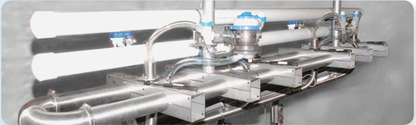
Stainless steel panels protect these critical components and allow for quick and easy cleanup.
